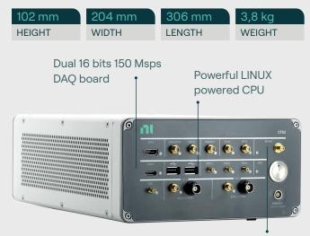
Full featured NFC tester with power amplifier reader / card emulation test / measurements conformance testing.
